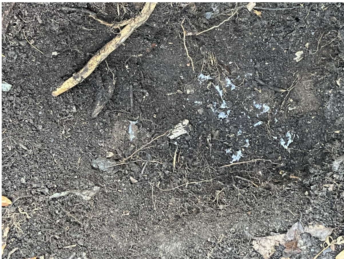
Figure 8 - Image showing burial site three on day of retrieval (2/12/21) showing retrieval couldn't be complete due to the paper being broken into many small fragments.
